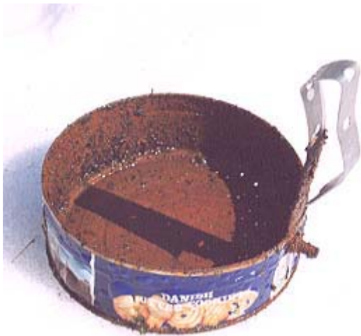
RIP! This is the sacrificial electrode. As you can see, the butter cookies are gone, as is the plating, parts of the label, and lots of metal.
